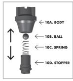
Dismantle valve by removing the stopper (10D), spring (10C) and ball (10B) from the body (10A).
